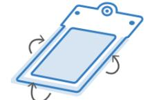
Fold up each side of the stabilizer and press it over the edges until it adheres to the frame.
