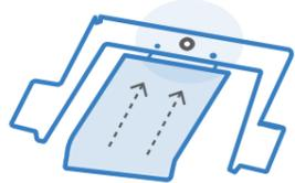
**5.** Insert the master bracket into the machine, as you would with a standard hoop. Note: Steps 3 and 4 are interchangeable. You can first place the garment over your hoop, and then insert the hoop into the master bracket, or first insert the hoop into the master bracket and then place the garment over your hoop and master bracket.
