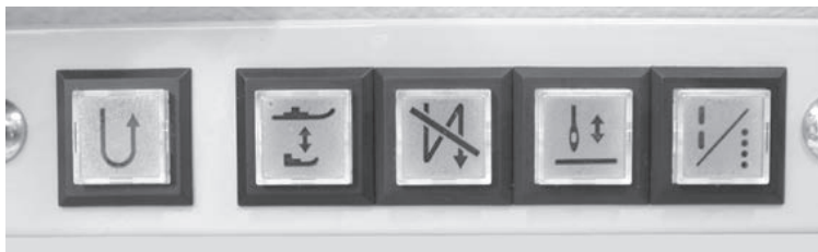
Simple setting for alternating presser foot movement
