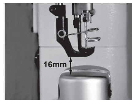
The clearance under the presser foot (16mm)
