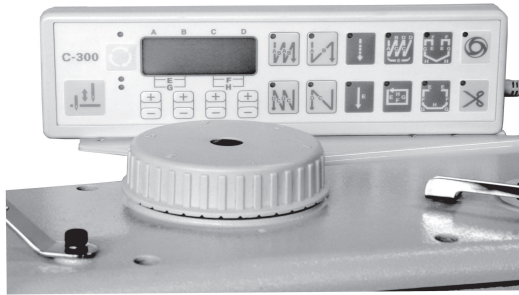
Simple setting for alternating presser foot movement
