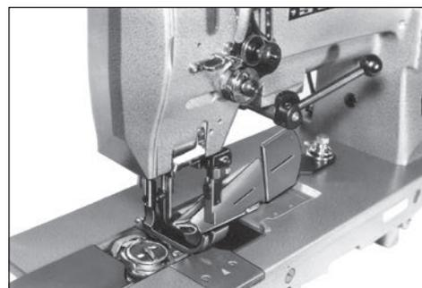
Suit for trimming and taping simultaneous for bedding, cover, cushion and carpet, etc. Trimming can be made in front of needle.
