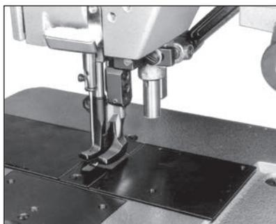
Suit for sewing and trimming simultaneous for leather, vinyl, heavy materials, automobile-interior, exterior decorations.
