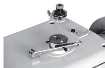
Built-in bobbin winder that enables simple and fine adjustment of winding volume of threads
