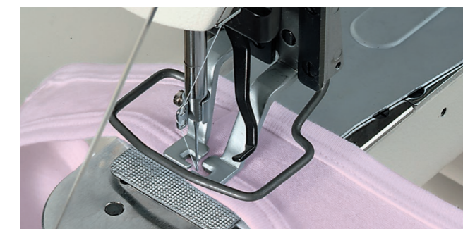
M type (Bartacking shoulder of running shirt)
