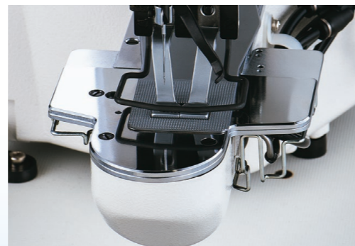
Bird's nest preventing /Shorter-thread remaining functions
