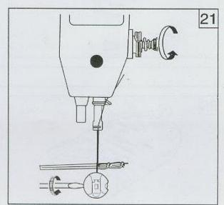
(B) The needle thread tension is too weak or the bobbin thread is too strong, turn the tension regulating thumb nut clockwise to make the needle thread get more tension or turn the bobbin case tension regulating screw counter clockwise with small plastic screw driver to make the bobbin thread get less tension (Fig.22)
