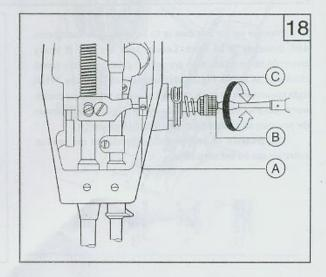
spring (C) to zero, and to turn tension stud (B) clockwise until spring (C) just comes into contact with the stop slot on the thread take-up spring regulator, then to further turn tension stud (B) counter-clockwise by 1/2 turn after adjustment, tighten tension stud set screw (A).
