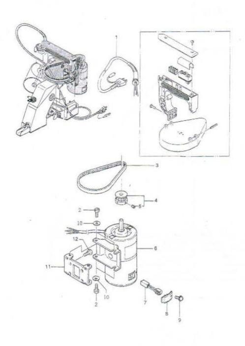
(6)MOTOR, PARTS (For totally Enclosed Type Motor)
