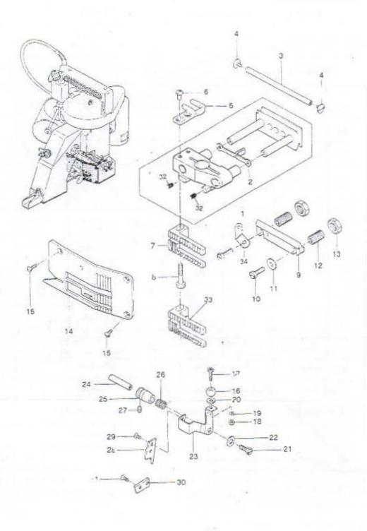
(5) FEED DRIVING AND THREAD CUTTER PARTS
